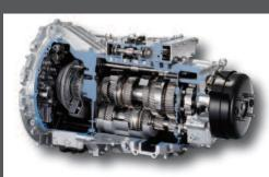
Duonic, the World's first truck dual clutch gearbox, drives like a full automatic but, like a manual, pulls heavy loads without heat build up. Its ECO mode provides additional fuel savings.
