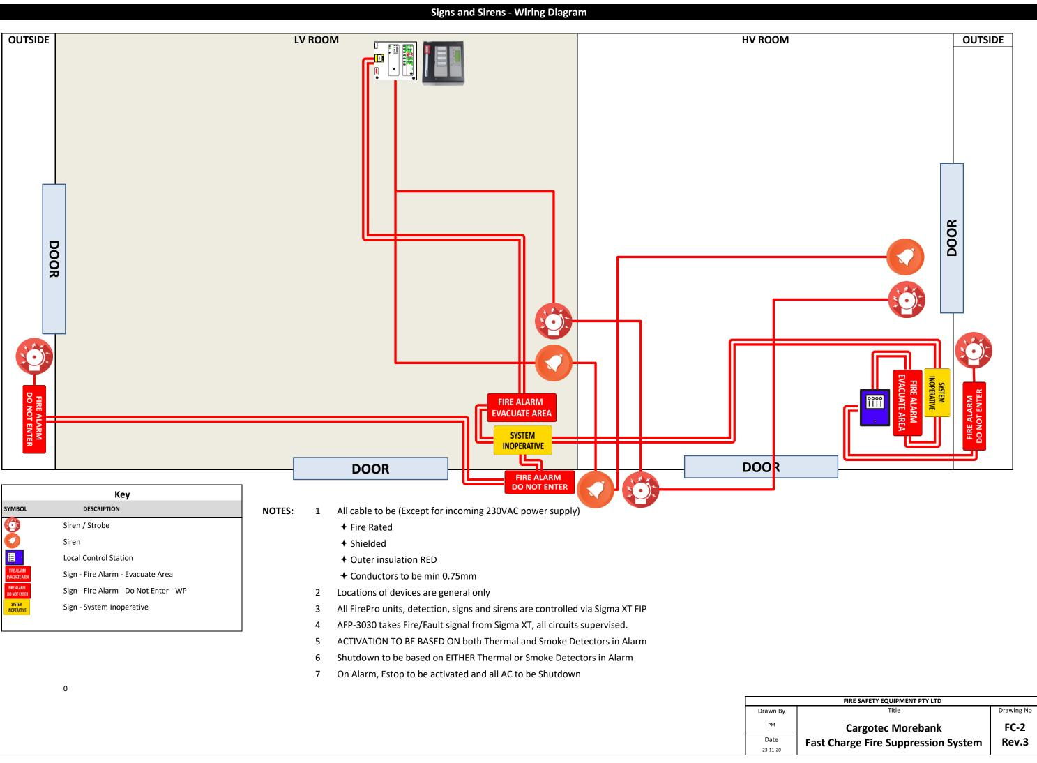
**Detection - Wiring Diagram**
