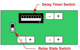
Each switch on the Delay Timer has a separate delay value (in seconds) as follows:
