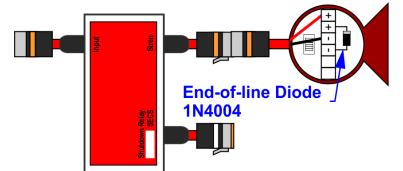
If not using a siren/strobe, the end-of-line diode should be terminated into the supplied 3 pin deutsch plug (note polarisation) and then connected to the "Siren" output on the module (marked orange). The end-of-line plug should then be covered in heatshrink, and the heatshrink crimped, to avoid ingress of water into the circuit.
