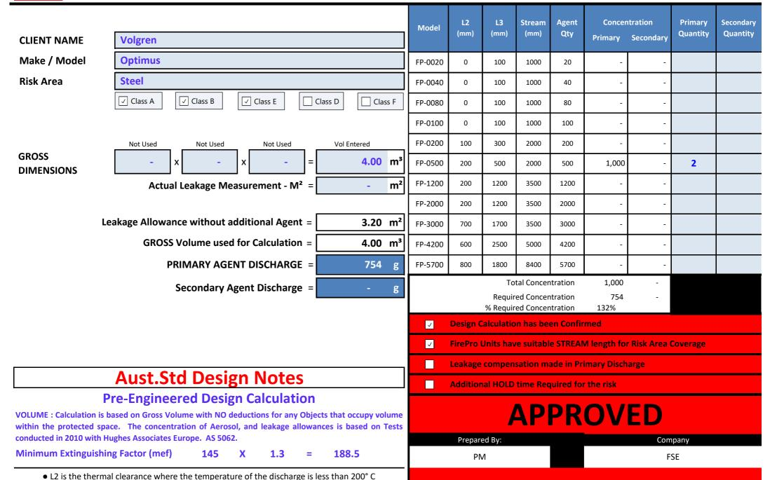
• L3 is the thermal clearance where the temperature of the discharge is less than 75° C
