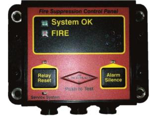
In isolation mode if either detection circuit is activated the red FIRE LED will illuminate, the audible alarm will sound, and the relay will begin countdown. This condition would remain until the source of the alarm is cleared.
