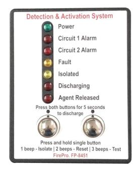
In isolation mode if either detection circuit goes into ALARM the LED will illuminate, the and NO audible alarm will sound. This condition would remain until the source of the alarm is cleared. The system should stay in isolation until the Alarm is cleared. If the isolation is turned off the system will activate.
